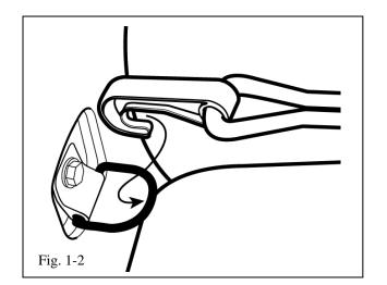
(b) Lay out the net so the zipper is on top and at the rear of the vehicle. Starting on the driver's side of the vehicle, attach the hook at the front of the net to the D-ring as shown (Fig 1-2).
